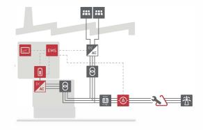
\* Two Power Conversion Systems (PCS), one MV transformer and Ring Main Unit (RMU), and one auxiliary cabinet and transformer are all integrated onto a single skid base.
